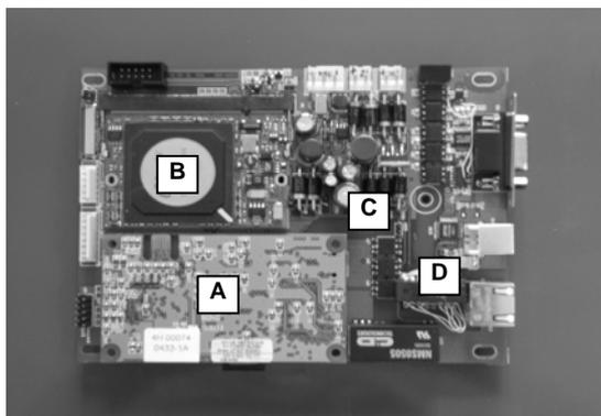
Fig. 1. Main board of the pulse oximomitor (A - Pulse oximeter module, B – PC Module, C - Galvanic separation, D - Communication interfaces)
