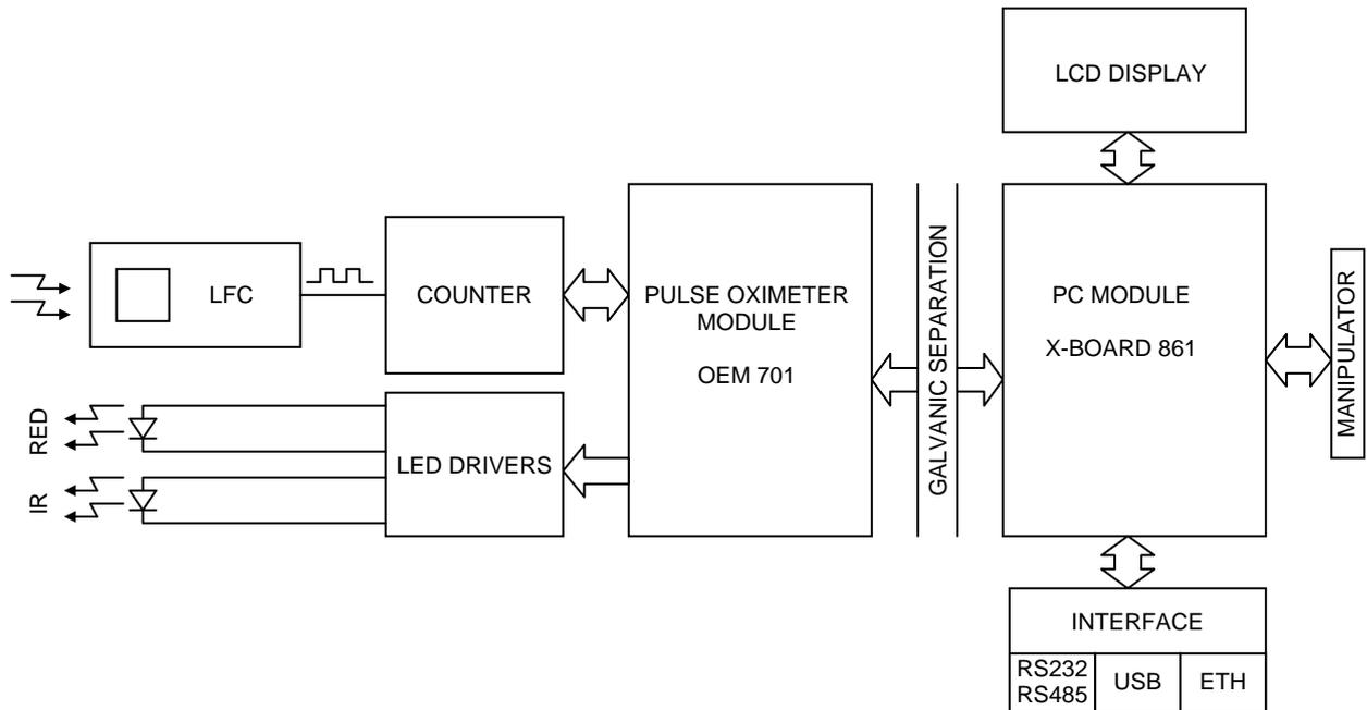
Fig. 2. Modular design of the pulse oximeter
