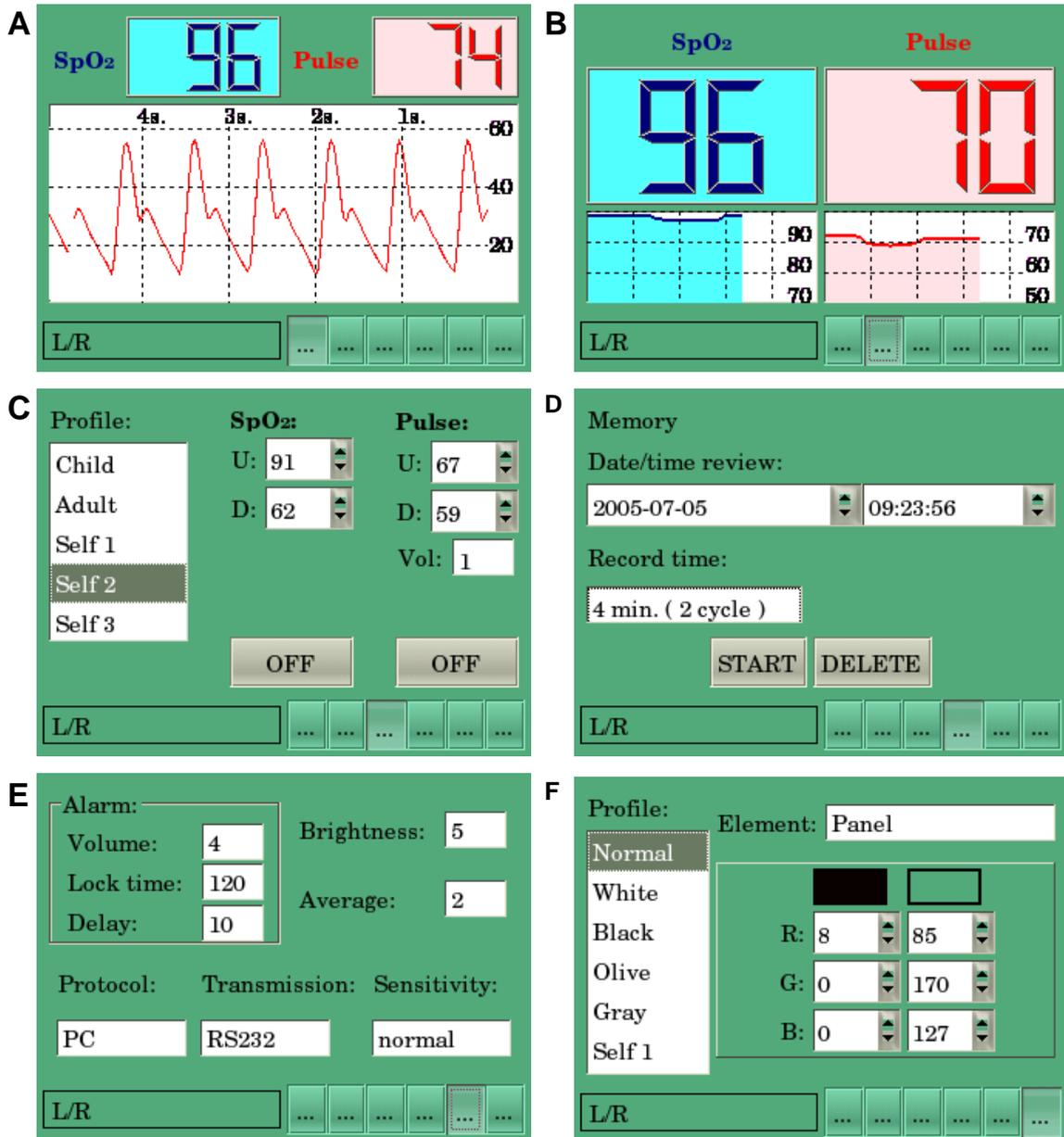
Fig. 4. Sample screens: the plethysmographic chart screen (A), SpO2 and Pulse charts screen(B), alarm configuration screen (C), chart browser screen (D), device configuration screen (E), color scheme configuration screen(F).
