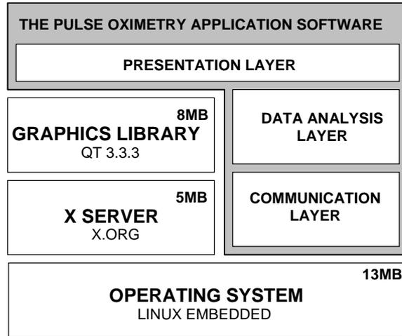
Fig. 3. Software architecture
