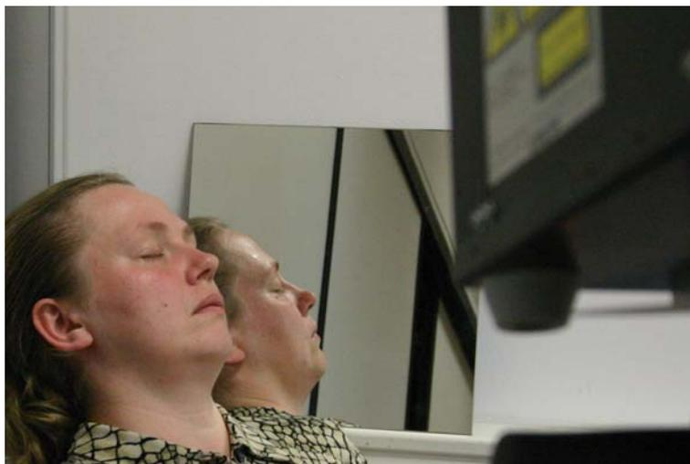
Fig. 8. Scanning a face simultaneously from the right (directly) and from the left (by scanning the “right” cheek of her mirror twin)
