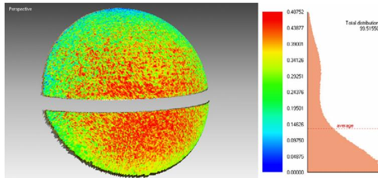
Fig. 3. Shell deviations for scans of a sphere
