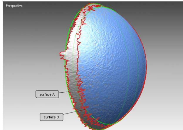
Fig. 7. Comparison of scans of a sphere with rejection of surfaces inclined less than  $20^\circ$  and without rejection
