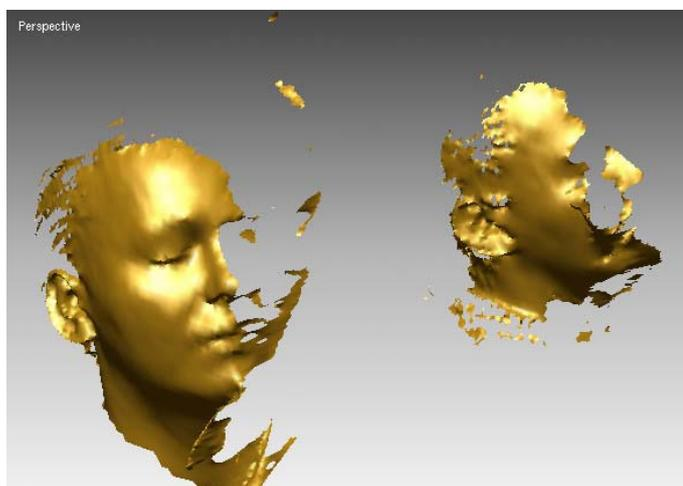
Fig. 9. 3D scans obtained with the mirror. Large artifacts protrude from the real person’s chin into the normally empty space in front of her left cheek. Note also the holes and deformities in the face of the “mirror twin”.
