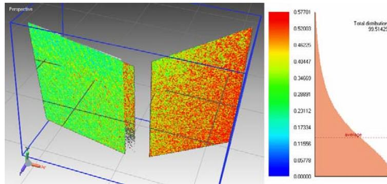
Fig. 2. Shell deviations for scans of planar surfaces
