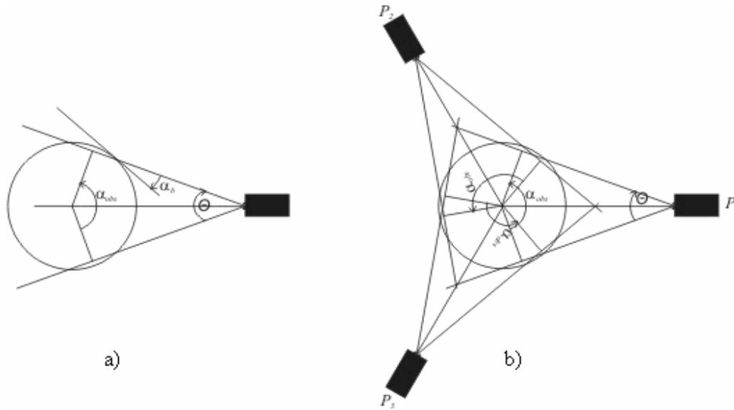
Fig. 6. Angular criteria for the rejection of steep surfaces (distance between object and scanner not to scale)
