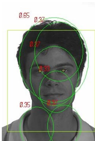
Fig. 1. A face image with detected ellipses. The numbers indicate the confidence of finding an ellipse. In the second step of the detection only one ellipse was classified by the SVM as a face and its eye positions are marked in the image.
