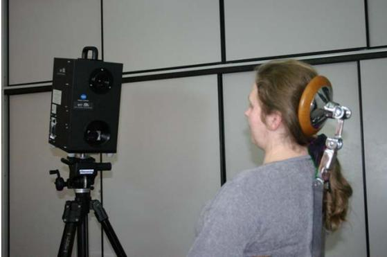
Fig. 3. 3D surface scanning system.
