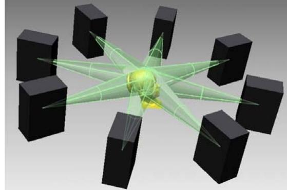
Fig. 4. Scanner viewpoints during acquisition of 3D surfaces.
